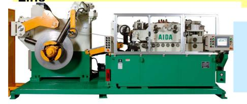
A Direct-Drive Loop-Free LFU Straightener Feeder
